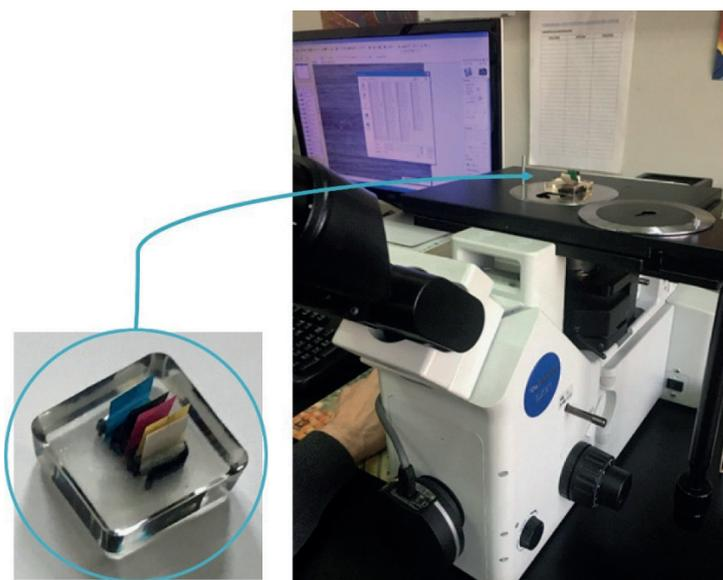
**Figure 1. The specimen inserted into an epoxy resin and light microscope Olympus GX 51 analysis of the cross section of samples**
