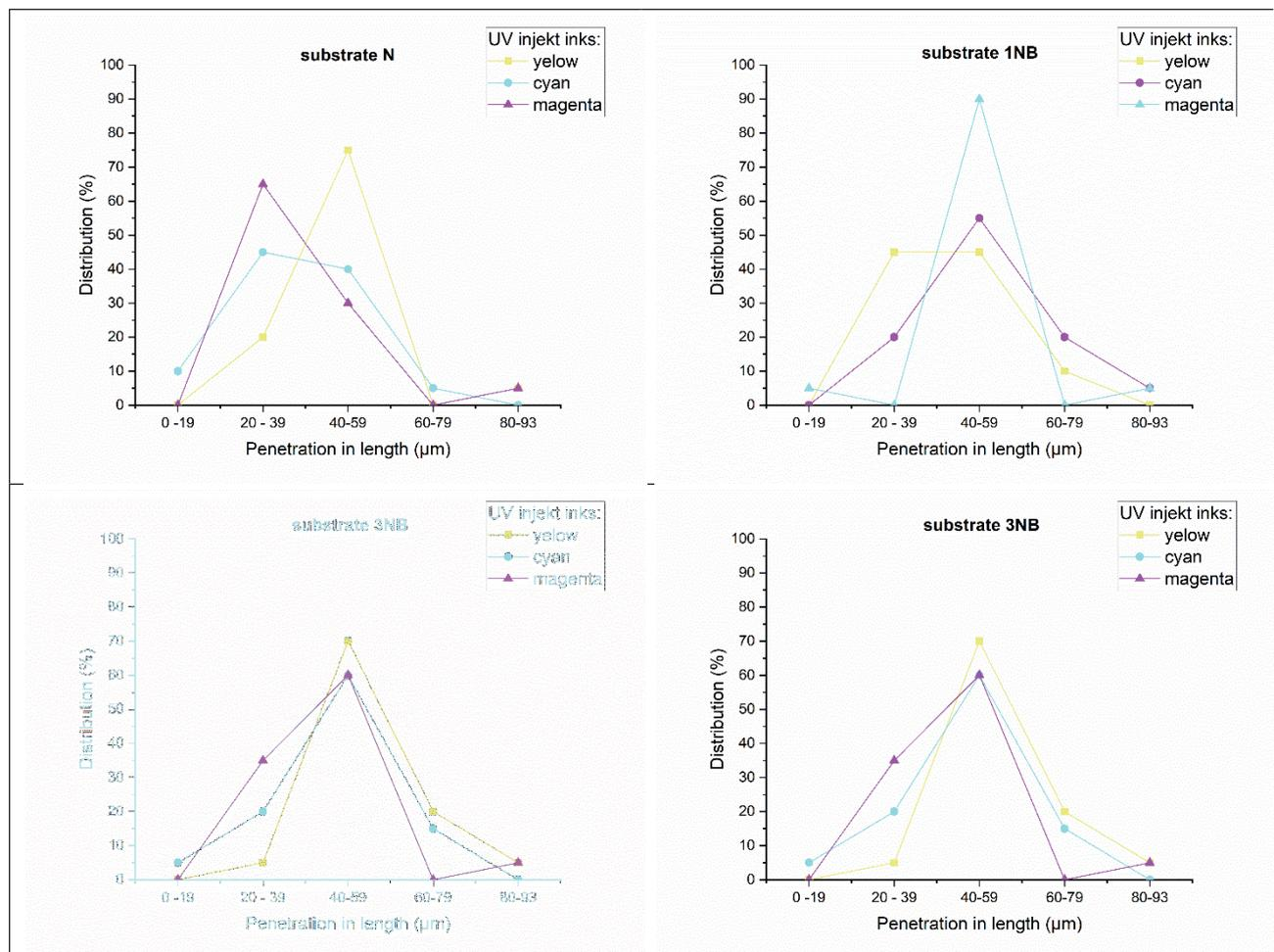
**Figure 3. Penetration results distributions of UV inkjet inks into laboratory substrates**
