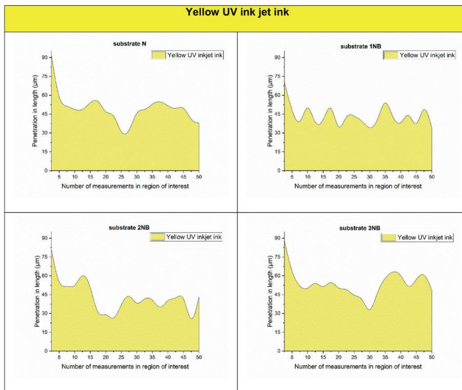
**Figure 6. Penetration profile of yellow ink into laboratory substrates**
