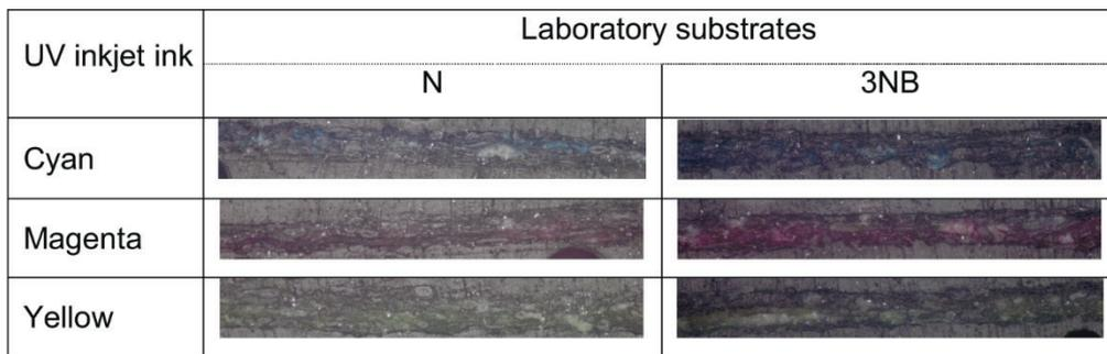
**Figure 2. Cross section of laboratory substrates N and 3NB printed with cyan, magenta and yellow ink**
