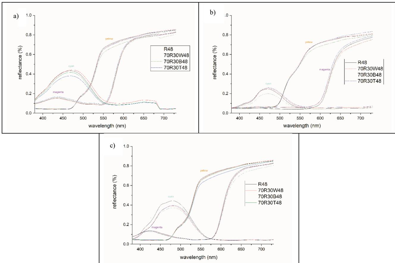
Figure 2: Reflectance values of cyan, magenta and yellow prints on laboratory paper substrates (R, 70R30W, 70R30B, 70R30T) produced by: a) offset printing process; b) gravure printing process; c) screen printing process after 48 hours of artificial aging
