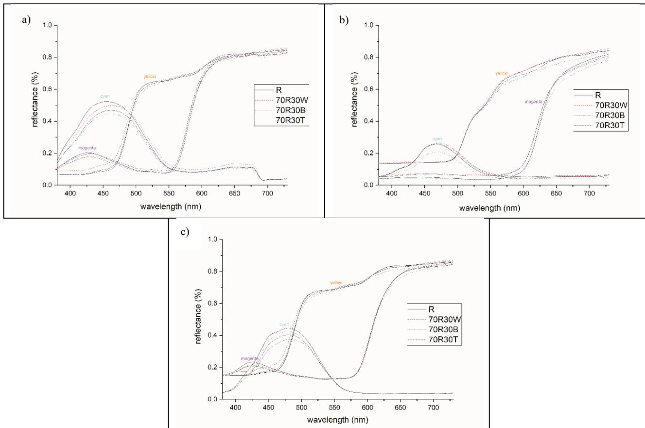
Figure 1: Reflectance values of cyan, magenta and yellow prints on laboratory substrates (R, 70R30W, 70R30B, 70R30T) produced by: a) offset printing process; b) gravure printing process; c) screen printing process
