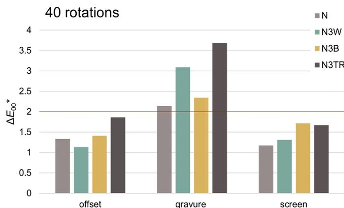
Figure 2: Comparison of color difference  $\Delta E_{00}^*$  of multilayer prints after 40 rotations of rub resistance test
