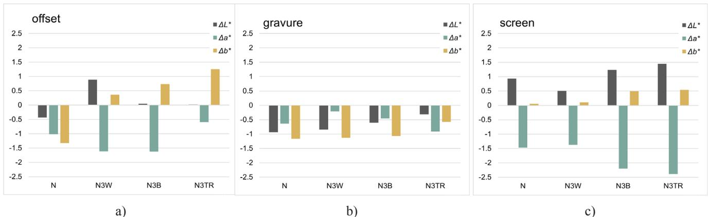
Figure 4: Difference  $\Delta L^*$ ,  $\Delta a^*$  and  $\Delta b^*$  before and after 60 rotations of rub resistance test for a) offset prints, b) gravure prints and c) screen prints
