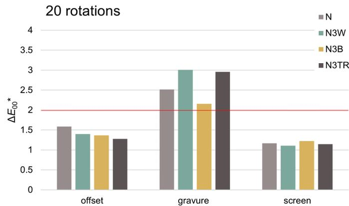
Figure 1: Comparison of color difference  $\Delta E_{00}^*$  of multilayer prints after 20 rotations of rub resistance test
