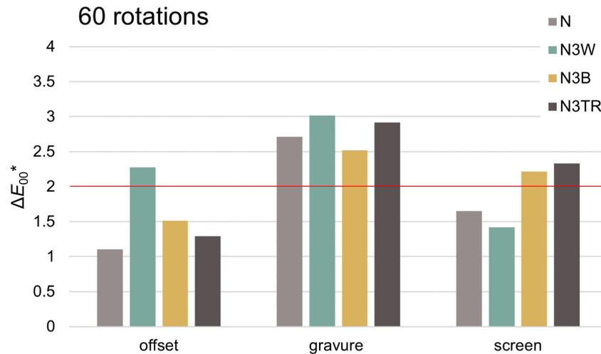
Figure 3: Comparison of color difference  $\Delta E_{00}^*$  of multilayer prints after 60 rotations of rub resistance test
